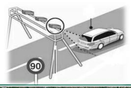
Radar–type: This type is mostly used in which the officer manually detects or installs the device in radar target the car and the waves reflect back to the receiver. The reflected wave from the target car changes in size or frequency. Then the detector will calculate the speed value of the car.
