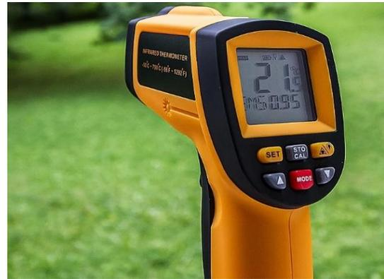
Infrared thermometers are tools used to quickly measure the surface temperature of an object without touching it. The infrared thermometers are used in wide range of applications including medical and industrial use. The measured temperature can range from 0-3,600 °C. The device takes in the radiation emitted by the object and calculates its temperature.
